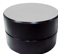
Leeb standard hardness block HLD-SB
